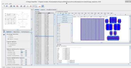
**AIDA-C** is the circuit-level synthesizer supported by state-of-the-art multi-objective optimization kernels, where the robustness of the solutions is attained by considering user-defined worst case corners, that account for process variations and(or) PVT corners. The circuit's performance is measured using **Spectre®**, **Eldo®** or **HSPICE®** electrical circuit simulators.
