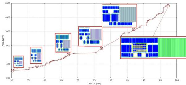
**AIDA-L** generates the complete layout of the sized circuit by placing and, routing the devices, while fulfilling the technology design rules by using built-in DRC and LVS procedures. The router takes into account the circuit's currents to mitigate electromigration and IR-drop effects, and a fast but accurate PEX procedure provides parasitic estimates to be used in **AIDA-C** layout-aware optimization.
